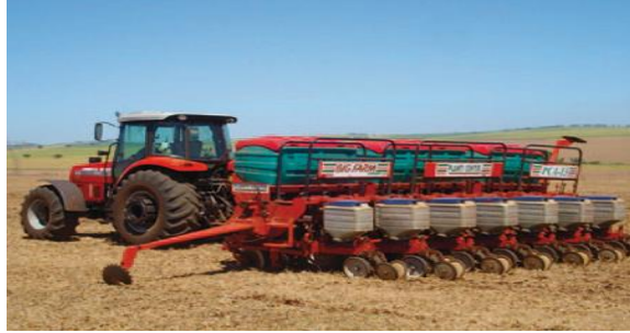
Fig. 4: Big farm seeder for direct seeding in crop residues, Floresta, State of Parana, Brazil.
