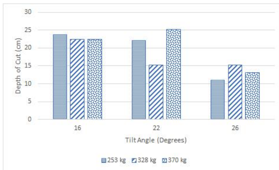
Figure 4: Effect of Implement Weight on Depth of Cut under varying Tilt Angle
