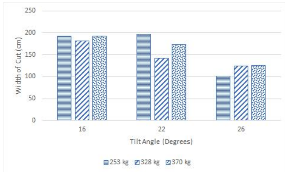
Figure 6: Effect of Implement Weight on Width of Cut under varying Tilt Angle
