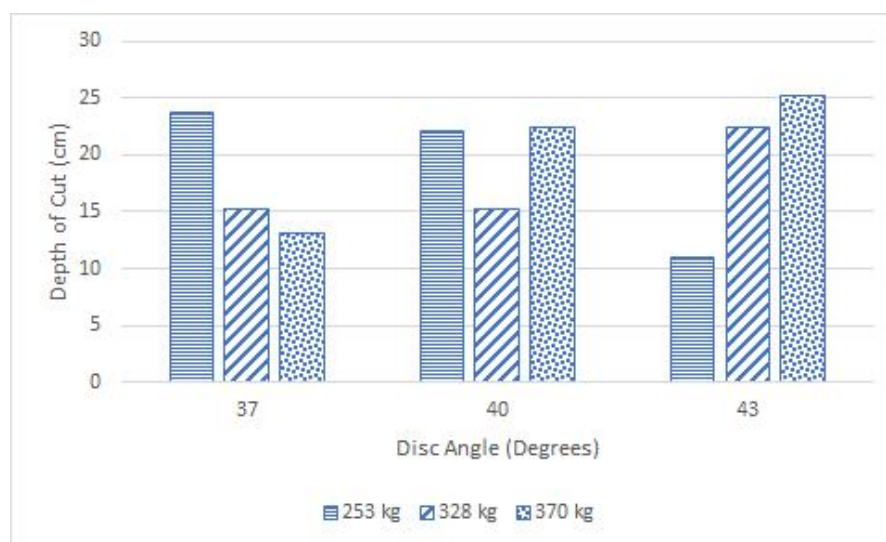
Figure 5: Effect of Implement Weight on Depth of Cut under varying Disc Angle
